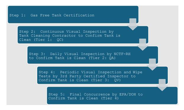
During any milestone of the inspection process, if there is doubt about reaching the SP-1 standard of tank cleanliness (whether through the QC, QA, or QV inspection process), NCTF-RH will direct the tank cleaning contractor to perform additional cleaning to meet the standards of SP1. Additional cleaning can range from spot cleaning with water at individual locations to completing additional pressure washing with Simple Green solution followed by additional freshwater rinsing.
